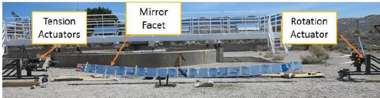
Figure 2. Image of small-scale Prototype 1 system. The horizontal distance over the cable span was about 9.1 m. The flat-plate receiver is located about 12 m to the right (not seen in the picture).
