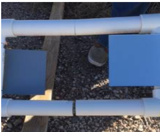
Figure 16. Prototype 2 ganged heliostat system under a 45° orientation demonstrating notable chaffing between adjacent facets at point of contact between upper PVC pipes pictured.
