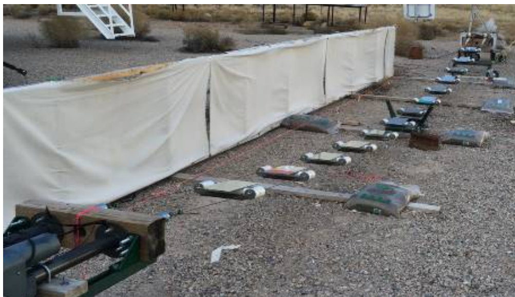
Figure 17. Prototype 3 with 13, 4 kg (9 lbs) facets, with a 9.1 m span and a 20:1 span to sag ratio, as well as with four respective clamps per facet.
