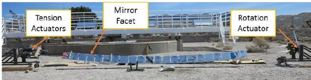
Figure 13. NSTTF ganged heliostat Prototype I installed at Sandia. Twenty-two mirrors, representing heliostats, are supported on two 1/8-inch guide wires.
