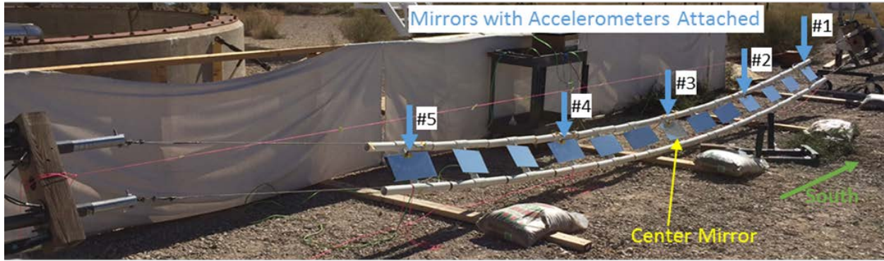
Figure 54. Prototype 2 set up with accelerometers attached to the five mirrors. In the Prototype 3 set up the same mirrors had accelerometers attached to them.
