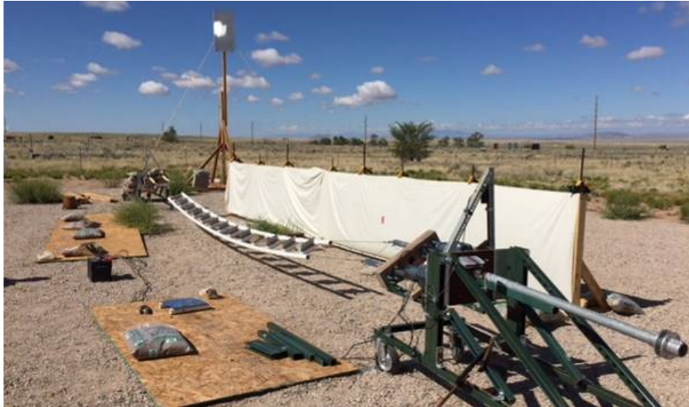
Figure 3. Image of Prototype 2 set up with a few mirrors put on-sun and the wind fence (covered with canvas tarp) to the west of the heliostat strip.
