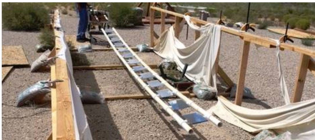
Figure 15. Experimental ganged heliostat Prototype 2, containing 13 rotatable facets.
